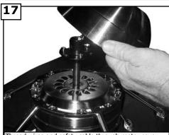
Thread wires and safety cable through motor cover.
